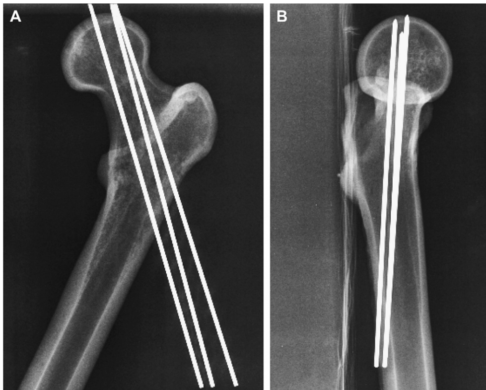
Figure 3 Fluorescent images showing the insertion of three pins in a Sawbones femur: (A) anteroposterior view; (B) lateral view.
